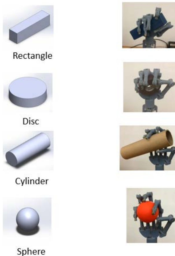
Fig. 5.8. Different grasps performed with hand according to the shapes of objects grasped
